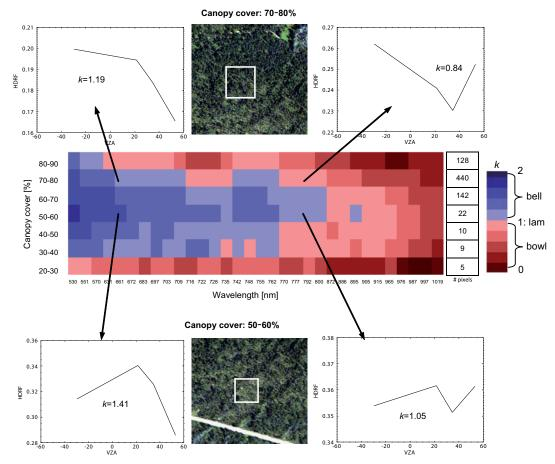
Figure 4.7: Averaged Minnaert-*k* values as a function of canopy cover and wavelength. The number of pixels per canopy cover class is given and some examples of the original angular signatures are shown. The RGB snapshots for a given canopy cover (white square) are derived from an HRSC (High Resolution Stereo Camera) acquisition in summer 2003. (lam= Lambertian)
