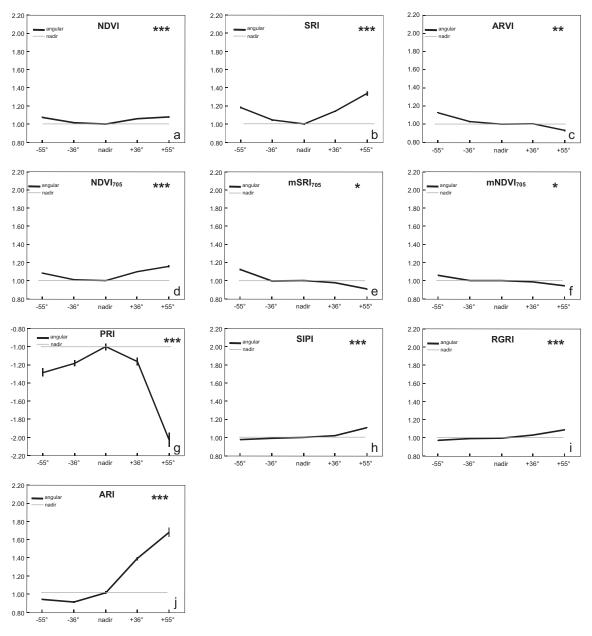
Figure 2.4: Averaged angular VIs values (normalized against its averaged nadir value) from forest reflectance values. *x*-axis denotes viewing angles (negative angles are in back-scattering direction, positive angles are in forward-scattering direction). *y*-axis denotes normalized VIs. The error bars shown are  $\pm 1$  SEM. Angular values were compared with nadir values by means of ANOVA RMs: significance levels: \*p < 0.05, \*\*p < 0.01, \*\*\*p < 0.001.
