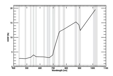
Figure 2.2: A typical canopy reflectance (438–1035 nm) of Swiss pine forest from the CHRIS sensor with its respective bandwidths (Mode 3).
