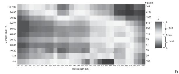
gure 5.4: Averaged Minnaert-k values as a function of canopy cover and wavelength. The numbers on the right represent the number of pixels for each class (lam= Lambertian).
