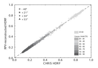
Figure 4.6: Comparison of CHRIS-HDRF and RPV-reconstructed HDRF at 631 nm for various canopy cover classes.
