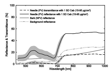
Figure 3.1: Averaged reflectance and transmittance of a PROSPECT-simulated needle, and reflectance of bark and background representing the spectral properties of PV, NPV, and background. The gray band represents the SD related to the *Cab* range of the needle.
