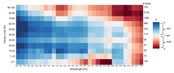
Figure 5.4: Averaged Minnaert-k values as a function of canopy cover and wavelength. The numbers on the right represent the number of pixels for each class (lam= Lambertian).
