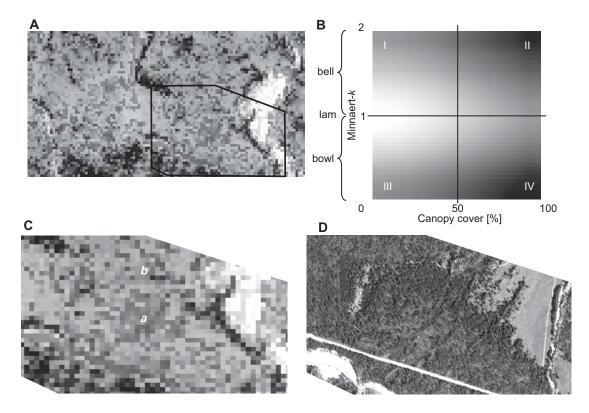
Figure 5.8: A) The RGB result of merging the Minnaert-k map with the canopy cover map. B) 2D color chart based on the color bar of the canopy cover map (*x*-axis) and the color bar of the Minnaert-k map (*y*-axis) (lam=Lambertian). C) Zoom-in of the merged map as presented in panel A. D) The reference image as derived from a high resolution stereo camera (HRSC) acquisition in summer 2003 (true color).
