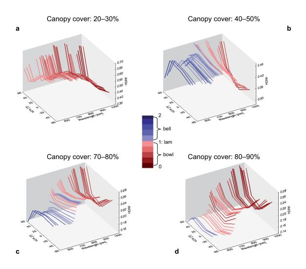
Figure 4.8: Averaged angular HDRF signatures for 4 canopy cover classes (a: 20-30%; b: 40-50%; c: 70-80%; d: 80-90%) with a color depending on the Minnaert-*k* value. Negative View Zenith Angles (VZA) represent the backscattering directions, positive VZAs represent forward scattering directions (lam= Lambertian).
