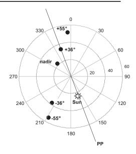
Figure 2.1: Polar plot of CHRIS image acquisition and illumination geometry as of June 27, 2004. PP: Principal Plane.
