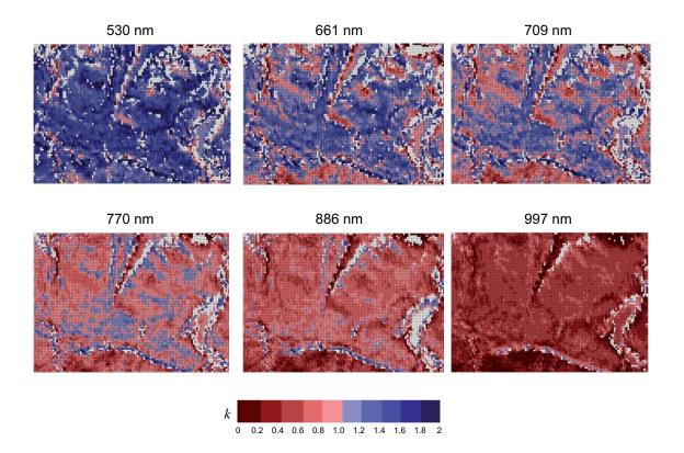
Figure 4.4: Minnaert-*k* maps for various CHRIS wavelengths. The white pixels are those in which the reflectance anisotropy of the CHRIS-HDRF data and the RPV-reconstructed HDRF data was significantly different.
