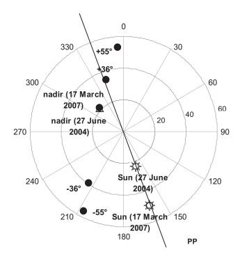
Figure 4.1: Polar plot of illumination geometry (Sun:  $\Leftrightarrow$ ) and CHRIS image acquisition as of March 17, 2007 (•), and nadir acquisition geometry as of June 27, 2004 ( $\Delta$ ). The nominal –55° view zenith angle missed the test site. PP: Principal Plane.
