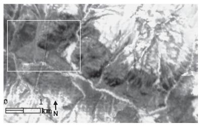
Figure 4.2: RGB subset of the geometrically and atmospherically corrected CHRIS/PROBA nadir scene acquired over the Swiss National Park study site on March 17, 2007. The Ofenpass valley stretches from upper left to below right of the image. The square indicates the core test site. The white part within the square is the snow-covered meadow. The pink color on the mountain tops is saturation effect. R: 631 nm, G: 550 nm, B: 442 nm.
