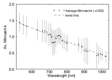
Figure 4.5: Average Minnaert-k and standard deviation as a function of wavelength. A linear trend line has been added.
