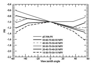
Figure 2.5: FLIGHT-simulated angular PRI values (normalized against their nadir value) for a coniferous forest. Viewing geometry is according to CHRIS FZAs ( $0^\circ$ ,  $\pm 36^\circ$ ,  $\pm 55^\circ$ ). Within-crown PV and NPV proportions varied with viewing angle (%NPV = 100 -%PV).
