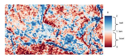
Figure 5.6: Minnaert-*k* parameter obtained by RPV model inversion at 722 nm (lam= Lambertian).
